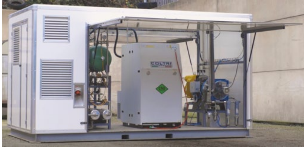
Mobile upgrading to Automotive grade biomethane
