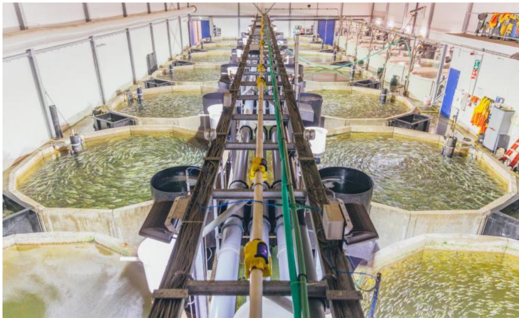
Figure 2: Picture of a fully enclosed - full recirculation RAS. Photo taken from Aquaculture Stewardship Council webpage (Anon, 2021)
