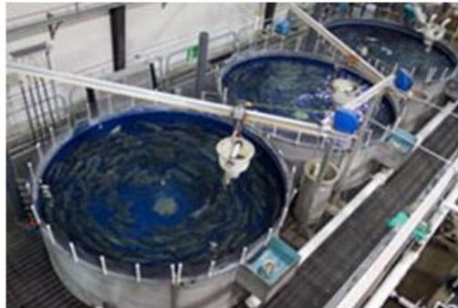
Figure 5: Picture of a partial recirculation RAS (Image taken from Freshwater Institute Website in Virginia)
