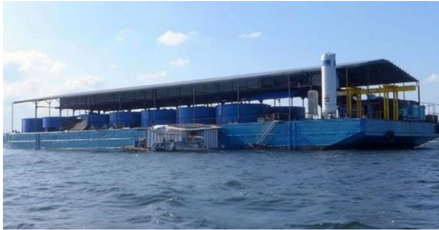
Figure 7: Picture of a marine floating full RAS (Image from Intrafish Technology 6 th August 2021)
