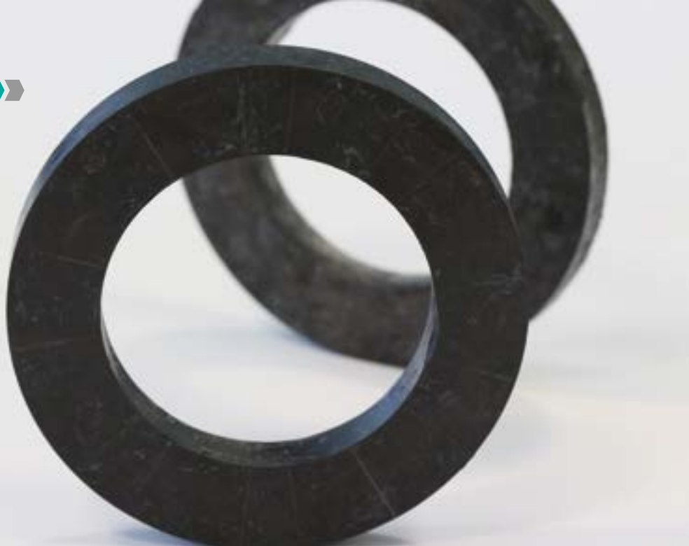
Left: Thermoplastic composite mouldings designed to replace aluminium alloys in aerospace applications.
