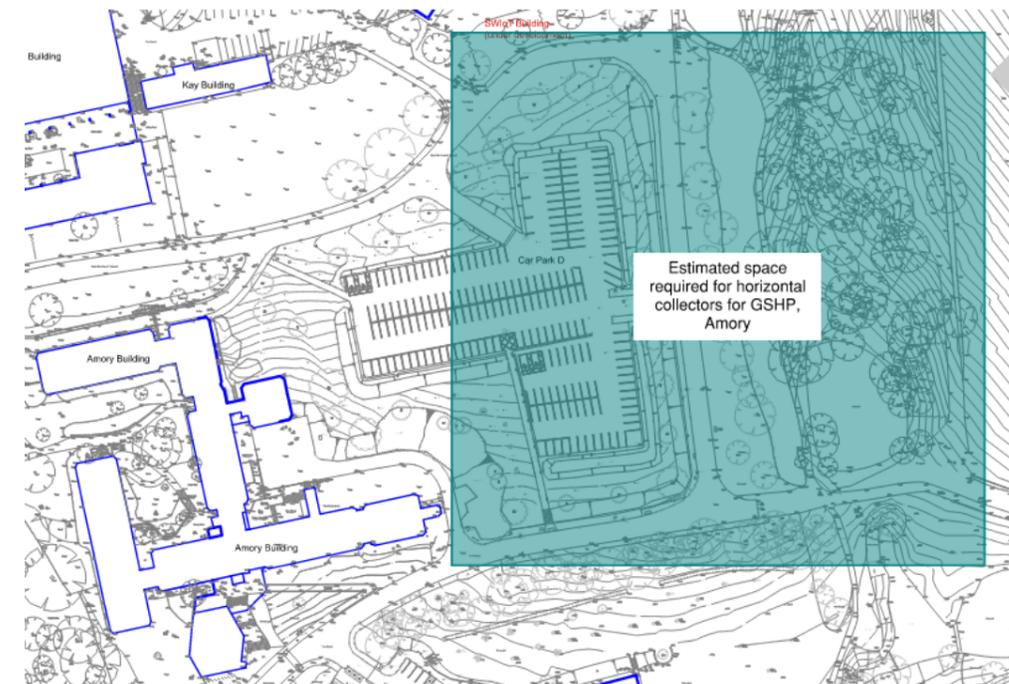
Figure 18: Estimated area needed for GSHP horizontal pipework for Amory building
