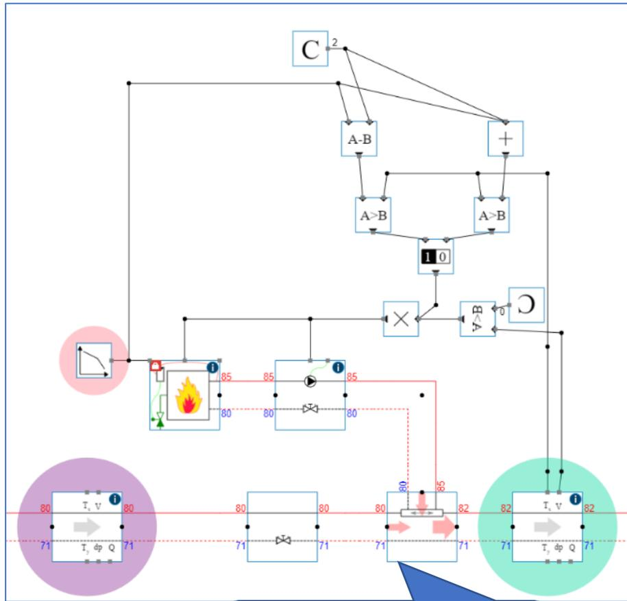
The shunt connection boosts the supply temperature to the asked heating curve set point
