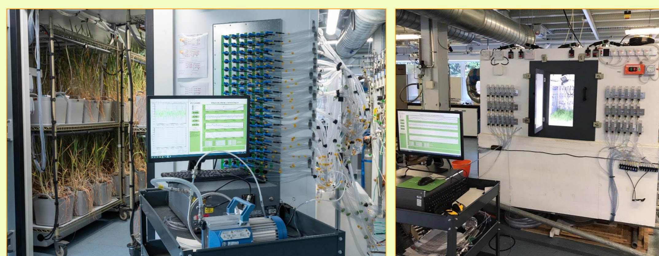
Fig. 1 ExSEQ growth chambers, equipped for continuous 13 C labelling and gas flux measurements
